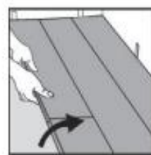
Step 7 Pull bar and rubber mallet can be used for final row of planks, ensuring a 5mm expansion gap
