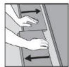
Step 8 Refitting of skirting board with hidden 5 mm expansion gap
